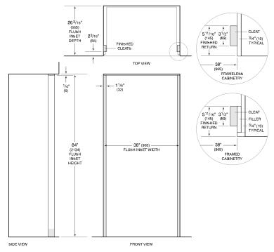
NOTE:  $3^{1}/e^{n}$  (89) finished returns and shaded areas will be visible and should be finished to match cabinetry. Shaded line represents profile of unit with  $3^{1}/4^{n}$  (19) panel.
