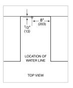
ICE MACHINE DRAIN lce machine models can be ordered with or without a drain pump. Models without a pump will drain water by gravity. A drain must be provided for all models.
