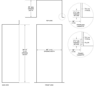
NOTE:  $3^{7}/2^{s}$  (89) finished returns will be visible and should be finished to match cabinetry.
