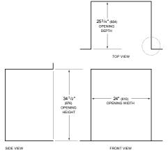
NOTE: 41/2" (114) finished returns will be visible and should be finished to match cabinetry
