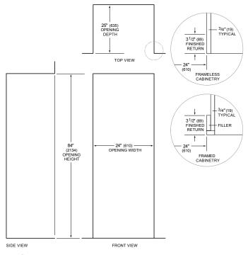
NOTE:  $3^{1}/2^{\circ}$  (89) finished returns will be visible and should be finished to match cabinetry
