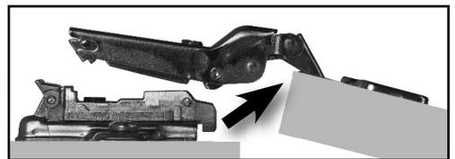
To re-install doors, line up hinges sliding hooks under pins (oval below).
