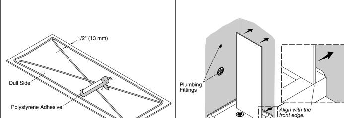
Cut the holes in the panel. Dry fit the panel and confirm hole locations.
