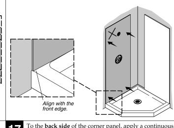
To the back side of the corner panel, apply a continuous 1/4" (6 mm) bead of panel adhesive 1/2" (13 mm) from the edge.
