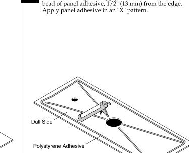
Adhesive toward the wall, install the panel to the wall with the plumbing fittings aligned as shown. Press firmly. Using a soft cloth, apply pressure and rub the entire surface.
