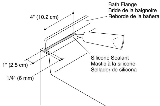
**NOTICE:** Silicone sealant must be applied before installing the end walls.
