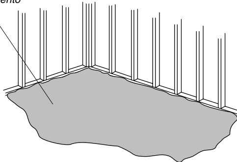
**NOTICE:** For best results, we recommend that you install a bed of mortar cement on the subfloor. This will not only provide solid support, but will also eliminate the potential for movement and noise when in use.
