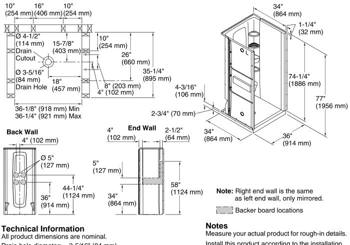
Drain hole diameter: 3-5/16" (84 mm) 29-3/16" x 32-3/4" (742 mm x 832 mm) Basin area, bottom: 29-3/16" x 32-3/4" (742 mm x 832 mm) Basin area, top: Weight: 96.4 lbs (43.7 kg) Door height required: 72-1/2" (1842 mm) Door width required: 32-3/4" (832 mm)
