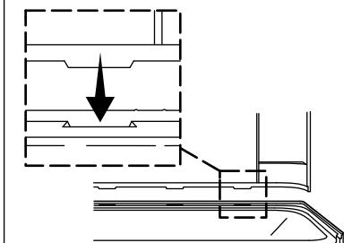
**14** Measure, mark, and drill the faucet holes in the end wall.
