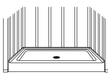
**7** With the unit level, shim under the support feet as needed.
