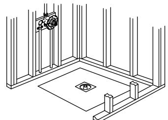
**5** Without a pad, set the basin area in 1" (25 mm) to 2" (51 mm) of mortar cement.
