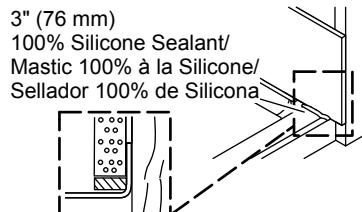
**12** Custom Walls: Install finished wall and 100% silicone sealant as shown. Leave weep channel open.
