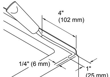
**16** STERLING Wall Sets with Dry-Block Seal: Verify that the seal is present, fully seated, and clear of debris.
