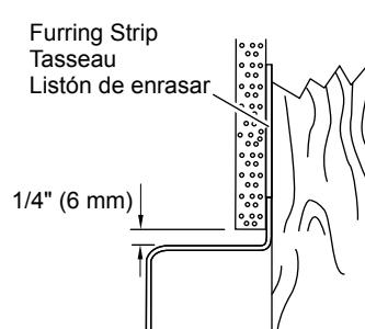
**11** Custom Walls: Apply 3" (76 mm) of 100% silicone sealant across threshold at front corners, below and flush with wallboard. Completely fill the void.
