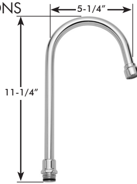
Spout -5, rigid or swivel 5-1/4" deep gooseneck
