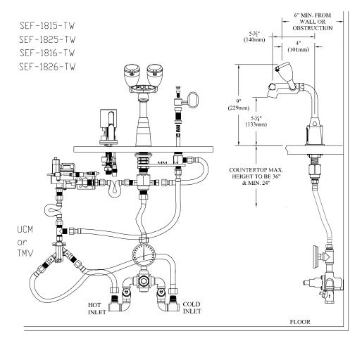
SEF-1815-TW -8" Sensorflow, eyewash faucet, UCM, MO, battery and Thermostatic Valve for Eyewash SEF-1825-TW -8" Sensorflow, eyewash faucet, UCM, MO, AC/DC and Thermostatic Valve for Eyewash
