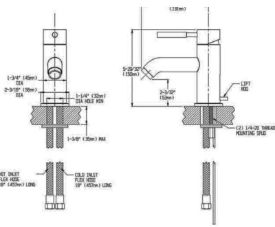
NOTE: 1. All dimensions are in inches (millimeters) unless otherwise specified and are subject to change without notice. 2. Flex hoses have 3/8 compression female threaded connections
