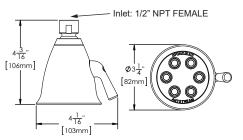
Model: SR-2256-E2 Max. Flow Rate: 2.0 gpm (7.6 L/min) Min. Flow Rate: 1.75 gpm (6.6 L/min) @ 45psi FOR USE WITH AUTOMATIC COMPENSATING VALVES RATED AT 6.6 L/MIN (1.75 GPM) OR LESS.
