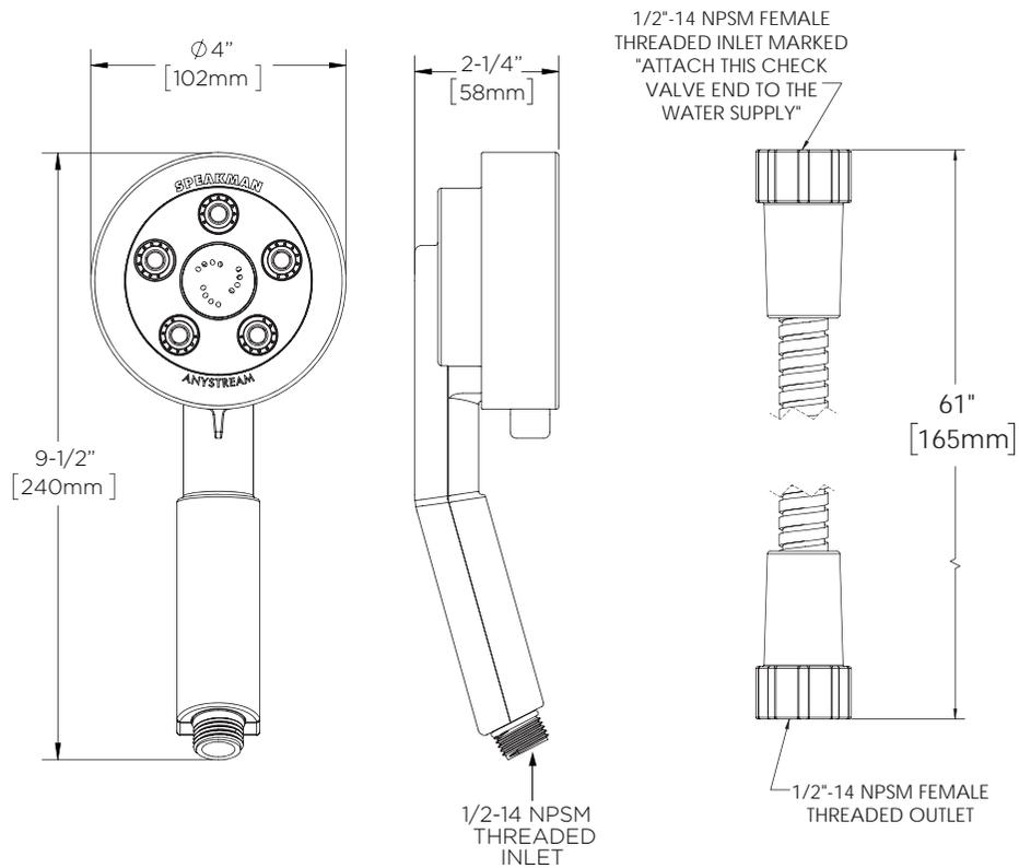
$1/2"$ -14 NPSM FEMALE THREADED INLET MARKED "ATTACH THIS CHECK VALVE END TO THE WATER SUPPLY"
