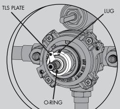
NOTE: A thermometer can be held at the Valve outlet to aid in either checking the existing factory setting or reaching the desired outlet temperature.
