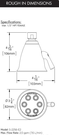
Max. Flow Rate: 2.0 gpm (7.6 L/min) Min. Flow Rate: 1.5 gpm (5.7 L/min) @ 45psi FOR USE WITH AUTOMATIC COMPENSATING VALVES RATED AT 6.6 L/MIN (1.75 GPM) OR LESS.
