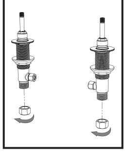
Remove Compression Nuts ① from End Bodies. Retrieve the Tee Assembly bag group. Slide a Compression Nut (1), followed by a Compression Sleeve (2) over the copper pipe of each end of the Tee Assembly.
