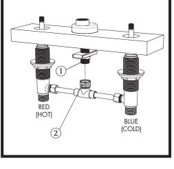
8 Ensure the Flange Nuts are flush with the tops of the 1-1/8"-16 UN threads, then tighten set screws ①.
