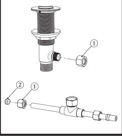
Bench assemble the Tee to the HOT and COLD end body valves. Be sure to fully seat the copper piping into the end body valves, and hand tighten Compression Nuts ① to the outlet ports. Be sure the end body valves are perpendicular to the Tee assembly.
