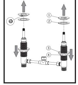
While lifting the end body with tee assembly up by its spindles, replace the rubber washers ① and screw the flange nuts ② back onto the end body valves, with flat side up, till they are flush with the tops of the 1-1/8"-16 UN threads of the end body valves.
