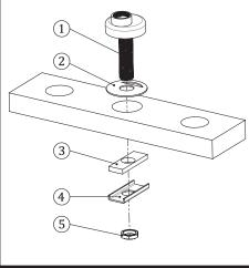
6 From below the counter top, push the end body with tee assembly up through the outer holes in the sink or counter top. NOTE: Blue colored end body (COLD) should be on the right side of tee assembly, Red colored end body (HOT) on the left. Hand tighten the tee assembly's swivel nut (2) to the shank of the gooseneck flange (1).
