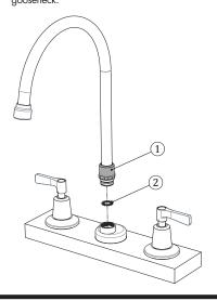
13 Turn on water supplies and flush both HOT and COLD cartridges for one minute, while checking for leaks. Once completed, install aerator into spout end using supplied aerator wrench.
