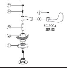
Assemble gooseneck to flange assembly by wrench tightening gooseneck collar nut (1). <u>NOTE:</u> For rigid gooseneck, place locking washer (2) from hardware bag group into flange outlet before assembling gooseneck.
