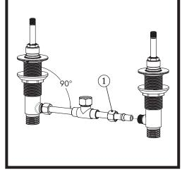
Loosen the set screws and remove the end body valve flange nuts ① and rubber washers② Screw the locknuts ④ and cup washers ③ down on end body valves.
