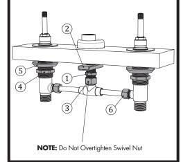
Insert and position the gooseneck flange ① with gasket ② down through the center hole of the sink or counter top, being sure the cut out of the gasket is aligned to the rear of the faucet. Assemble Rubber Washer ③, Metal Channel Washer ④ and Mounting Nut ⑤ to shank and thread only half way up the shank.
