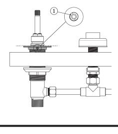
10 Connect water supply lines to inlets (1/2"-14 NPSM male threads) of the end body valves and wrench tighten coupling nuts to prevent leaks.
