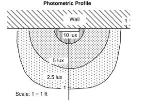
Measured 18" below bottom of the Guidelight (floor level)
