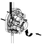
Remove filter from solenoid caddy assembly.
