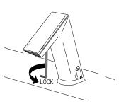
Rotate solenoid assembly counterclockwise through a 45° angle.
