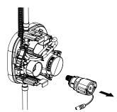
Insert solenoid caddy assembly into control module lining up arrows. Turn solenoid caddy assembly clockwise 45°.
