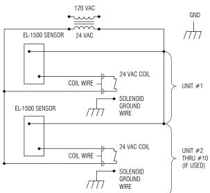
One Transformer serves up to ten (10) OPTIMA Closet/Urinal Flushometers. Specify number of transformers required accordingly.
