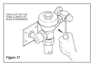
Important: DO NOT install the Cap onto the Sleeve unless the Sleeve has been threaded onto the Control Stop Bonnet. If assembled when off of the Control Stop, the Sleeve WILL NOT come apart from the Cap.
