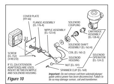
Solenoid Coil and Transformer.
