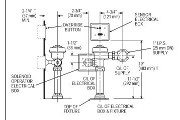
MODEL 115 ES-S — Water Saver, 3.5 gpf (13.2 Lpf) MODEL 115-1.5 ES-S — Low Consumption, 1.6 gpf (6.0 Lpf) MODEL 116 ES-S — Water Saver, 3.5 gpf (13.2 Lpf) MODEL 116-1.5 ES-S — Low Consumption, 1.6 gpf (6.0 Lpf)
