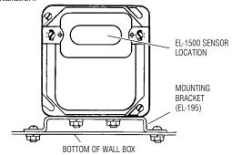
Adjust the Mounting Bracket so that the Sensor sits flush against the Cover Plate. Refer to the instructions packaged with the Flushometer for additional installation information.
