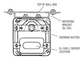
Adjust the Mounting Bracket so that the Sensor sits flush against the Cover Plate.
