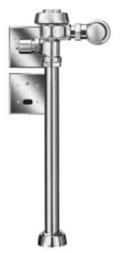
The Model 116 ES-S valve is designed for installations where the water supply is roughed in 27" (675 mm) above the top of the water closet. When installing the Model 116 ES-S valve, the electrical box for the sensor must be installed as shown on the back page of this sheet. Failure to install this valve properly will result in user complaints.
