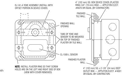
To ensure a perfect rough-in, Sloan recommends the use of the EL-485-A Flushometer Electrical Box Positioning and Support Kit. Specify and order the EL 485-A Kit separately. Consult factory for installation details.
