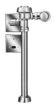
The Model 115 ES-S valve is designed for installations where the water supply is roughed in 24" (610 mm) above the top of the water closet. When installing the Model 115 ES-S valve, the electrical box for the sensor must be installed as shown on the back page of this sheet. Failure to install this valve properly will result in user complaints.
