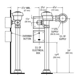
Position of Sensor Box can be raised or lowered 1" (25 mm) if in conflict with Handicap Grab Bars.
