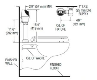
When installing the G2 Optima Plus in a handicap stall: Per the ADA Guidelines (section 604.9.4) it is recommended that the grab bars be split or shifted to the wide side of the stall. If grab bars must be present over the valve, use the Alternate ADA Installation as shown to the right.
