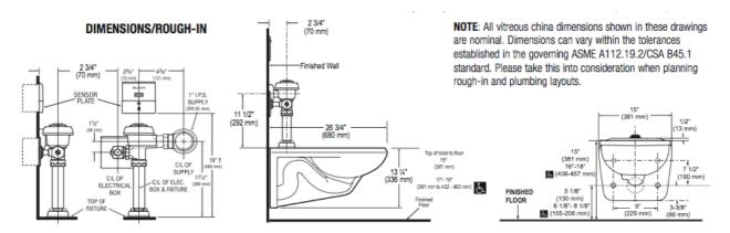
† Position of Sensor Box can be raised or lowered 1" (25 mm) if in conflict with Handicap Grab Bars.
