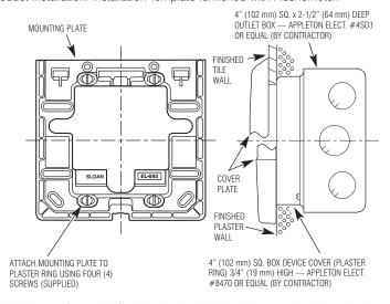
To ensure a perfect rough-in, Sloan recommends the use of the EL-485-A Flushometer Electrical Box Positioning and Support Kit. Specify and order the EL-485-A Kit separately. When using the EL-485-A kit, the Solenoid Plate roughs in at the Urinal location. Consult factory for installation details.
