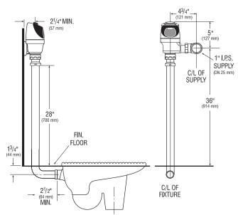
The Model 8137 no longer requires the use of a Beam Deflector to properly target the user
