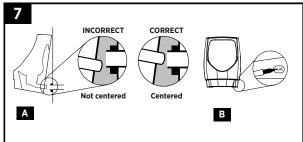
A. Hang bowl on the bracket and check tail pipe alignment, then remove the bowl and adjust the bracket as needed. Re-hang and re-check bowl alignment with the drain line. Tail pipe should align with center of drain line.
