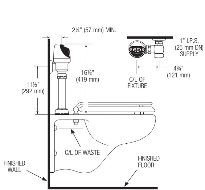
When installing the Sloan ECOS<sup>®</sup> Electronic in a handicap stall:
