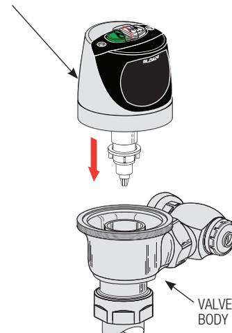
To facilitate installation, the O-ring on the diaphragm assembly must be wet for easier insertion. NOTE: Sensor Lens must face directly forward. Rotating the Sensor to either side will decrease the Sensor's ability to detect a target.
