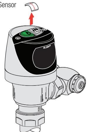
Important: The Locking Ring must be installed down past the valve body threads by at least one thread. If difficulty is experienced installing the Locking Ring, turn the Locking Ring back and forth, each time working it further down the threads. The Locking Ring will act as a thread chaser in the event there has been a build-up of matter on the threads of the old valve body.
