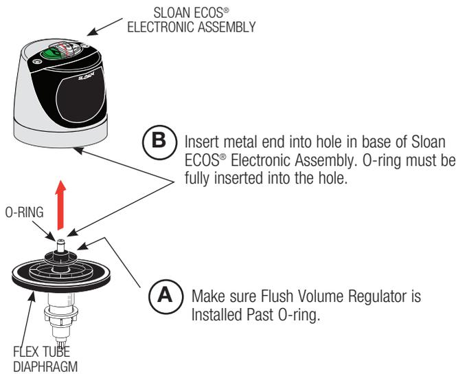
**C** Push Diaphragm securely against underside of Sloan ECOS® Electronic Assembly. Place entire Assembly onto the Valve Body.
