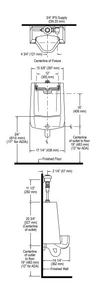
NOTE: All vitreous china dimensions shown in these drawings are nominal. Dimensions can vary within the tolerances established in the governing ASME A112.19.2/CSA B45.1 standard. Please take this into consideration when planning rough-in and plumbing layouts.
