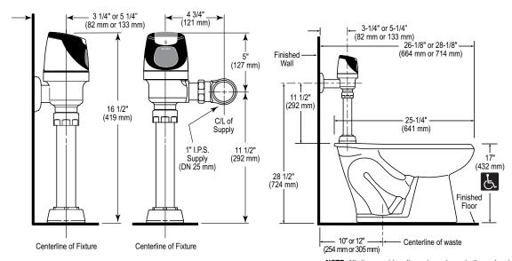
**NOTE:** All vitreous china dimensions shown in these drawings are nominal. Dimensions can vary within the tolerances established in the governing ASME A112.19.2/CSA B45.1 standard. Please take this into consideration when planning rough-in and plumbing layouts.
