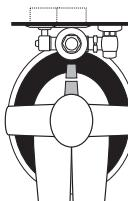
2. As the user enters the beam's effective range (15" to 30") the beam is reflected into the OPTIMA® Scanner Window and transformed into a low voltage electrical circuit. Once activated, the Output Circuit continues in a "hold" mode for as long as the user remains within the effective range of the sensor.
