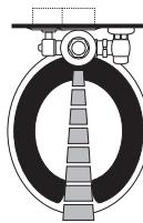
3. When the user steps away from the OPTIMA® Sensor, the circuit immediately initiates an electrical "one-time" signal that operates the Solenoid. This initiates the flushing cycle to flush the fixture. The Circuit then automatically resets and is ready for the next user.
