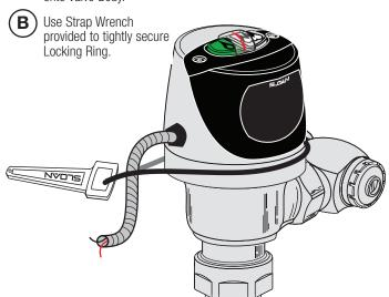
Important: The Locking Ring must be installed down past the valve body threads by at least one thread. If difficulty is experienced installing the Locking Ring, turn the Locking Ring back and forth, each time working it further down the threads. The Locking Ring will act as a thread chaser in the event there has been a build-up of matter on the threads of the old valve body.
