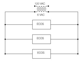
One EL-386 Transformer serves one (1) Optima Closet/Urinal Flushometer. One EL-451 Transformer serves up to eight (8) Optima Closet/Urinal Flushomteres.
