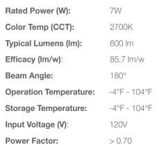
THD: 40% **Ignition Time:** Instant-On Line Frequency: 60 Hz Dimmable: No **Safety Certification:** c UL us **Energy Star Listed:** No E26 Base / Cap: **Product Life** 15,000 Hrs.
