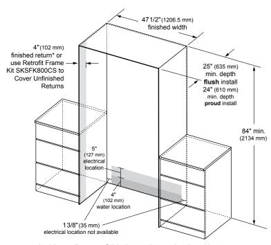
\*A minimum 4" (102 mm) finished return that matches the cabinet exterior is recommended on all sides and the top of the cutout opening. The shaded area will be visible after installation.
