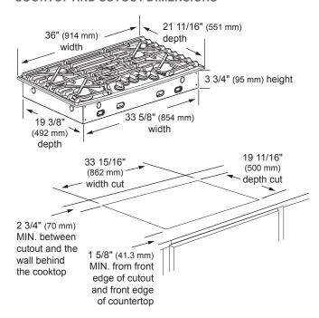
To ensure accuracy, it is best to make a template when cutting the opening in the counter
