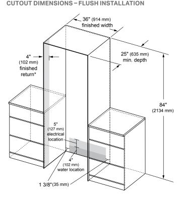
\* A minimum 4" (102 mm) finished return that matches the cabinet exterior is recommended on all sides and the top of the cutout opening. The shaded area will be visible after installation.
