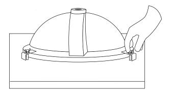
8. Wipe away any excess sealant with a damp cloth, and allow the sealant to dry. Once the sealant is dry, proceed to Step 3.
