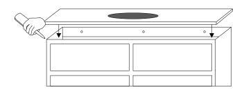
2. With assistance from another person, slowly and carefully set the counter top onto the vanity cabinet. Once positioned, press firmly into place. Wipe away any excess sealant using a damp cloth.
