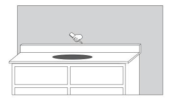
4. Allow the silicone sealant to dry, which could take up 24 hours.
