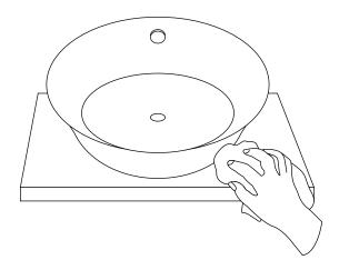
5. Let the assembled vanity sit for 24 hours to allow all the silicone sealant to fully dry. Once dry, proceed to the installation of your faucet and drain assemblies.
