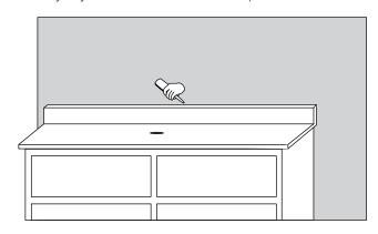
4. Allow the silicone sealant to dry, which could take up to 24 hours.
