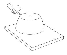
2. Turn the sink right-side-up and position over the 2" drain hole.
