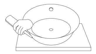
4. Remove any excess sealant to complete the sink installation.
