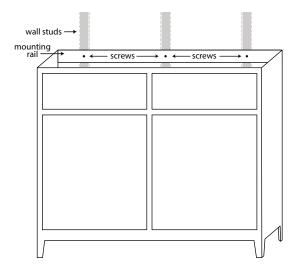
5. Attach the vanity to the wall by screwing through the mounting rail in the back of the vanity cabinet into the wall studs.
