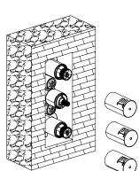
3. When the finished wall is complete, remove the protective covers.
