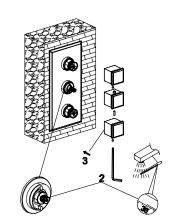
4. Install the escutcheon, and handle. Tighten the set screw with an Allen wrench to secure.
