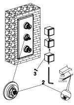
4. Install the escutcheon, and handle. Tighten the set screw with an Allen wrench to secure.
