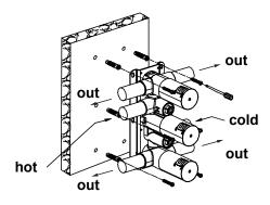
1. Install the valve body. Wrap the threaded portion of the joints in Teflon tape and connect the water inlet and outlet.
