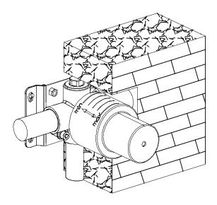
2. Put the protective cover on the valve body and finish the shower wall.
