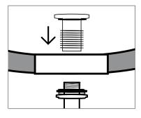
5. On the underside of the counter, attach the tapered rubber gasket. With the flat side facing down, slide the gasket up the threaded shank until it makes contact with the bottom of the sink.
