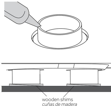
2b. If using mortar, press the shower base into place while the mortar is still wet. Be sure to apply weight (full water buckets work well) to the tray to ensure proper adhesion. Allow mortar to fully cure before proceeding further.
