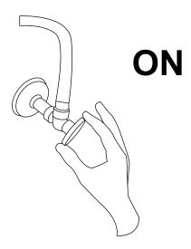
6. Remove the aerator from the spout. Turn the faucet on and allow the water to flow for approximately 60 seconds. Ensure that there are no leaks, and that both hot and cold water are running properly. Divert water to the sprayer setting and allow it to flow for another 60 seconds.
