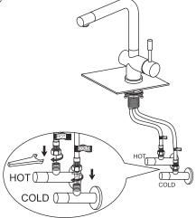
5. Once installation is complete, turn the main water supply back on from underneath your sink. Check for any leaks underneath.
