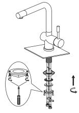
4. Apply plumber's tape or thread sealant to the threading on each of the faucet's water lines, and connect the main water hoses to the faucet. Ensure that you are connecting the hot and cold lines appropriately.
